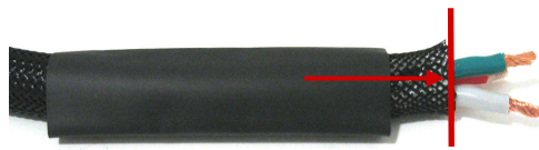
Fig.3: Pull sleeving straight until overhangs cable jacket 3/4"(in) ... then insert \text{Ø}3/4 "(in) x 3-1/2"(in) long heat shrink over cable until flush with sleeving edge
