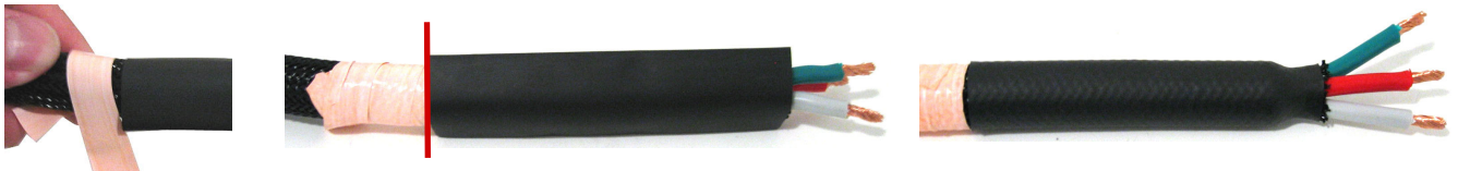
Fig.4: Wrap Teflon® tape around PET Techflex sleeving by starting at edge of heat shrink sleeving ... then shrink in place
