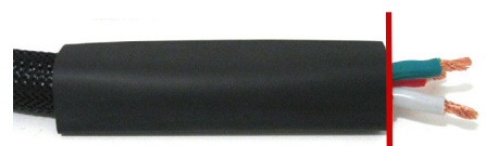
Fig.3: Pull sleeving straight until overhangs cable jacket 3/4"(in) ... then insert \text{Ø}3/4 "(in) x 3-1/2"(in) long heat shrink over cable until flush with sleeving edge
