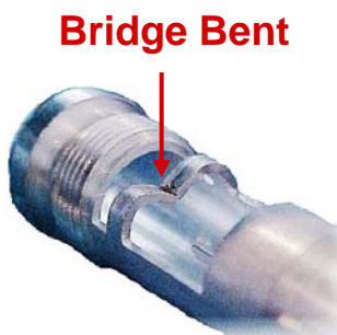
Fig.8: Bent Bridge for Copper Shield
